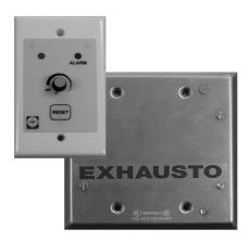
If the red LED flashes and buzzer sounds, the follwoing may have occured: defective chimney fan, blocked flue or disconnected power supply. The control can be reset, and the alarm turned off, by pressing the reset button for 1-2 seconds.
