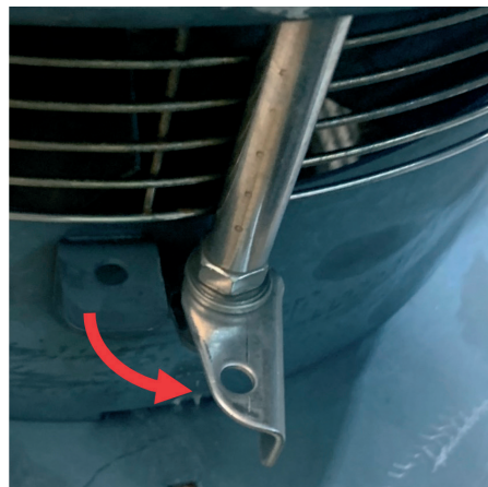
3 Remove fan head from base Using a 13mm wrench (bolt head) and 1/2" socket (nut).
