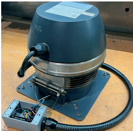
1 Switch OFF and tag out the power supply for the fan.
