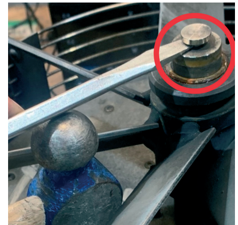
4 In order to remove the vane plug, loosen the setscrew using a 3mm Allen wrench. Pry up on the plug with a flathead screwdriver or clamshell style puller if necessary.
