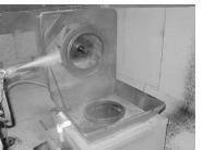
6.) It is very important to clean the impeller. If the impeller is only partly cleaned, it will be unbalanced. This will lead to vibrations and motor failure.
