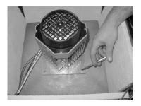
5.) Mount motor cover back onto fan and switch power back on.
